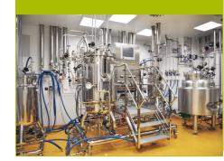
Reactors and storage tanks, filling lines, packaging lines, liofilizators, tableting machines, homogenizers.
